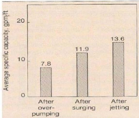
The graph above shows clearly the impact on specific capacity when overpumping was followed by surging, and then surging was followed by jetting. Specific capacities of the wells involved in this controlled test were improved
