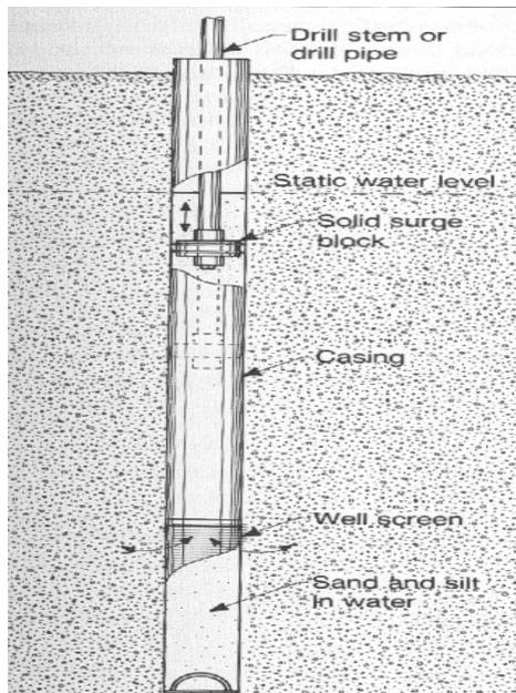
For removal of the sediment, the water/sediment mixture is allowed to exit the well at the ground surface
