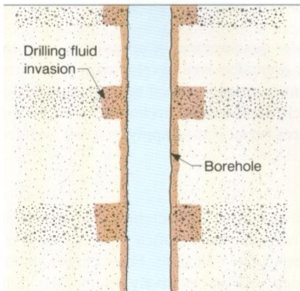
Well development removes fine sediments along the well screen-aquifer contact and some distance into the formation.
